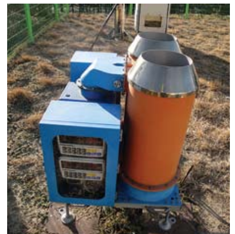
■ Automatic Cloud Observation instrument (left) and precipitation measuring system (right)
