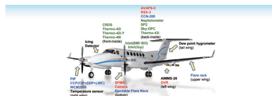
Instruments mounted on the aircraft
